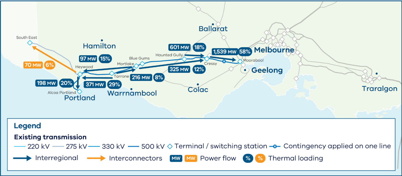
Figure 21 500 kV flows and loadings in South West Victoria post-contingent for Cressy-Moorabool line 1
