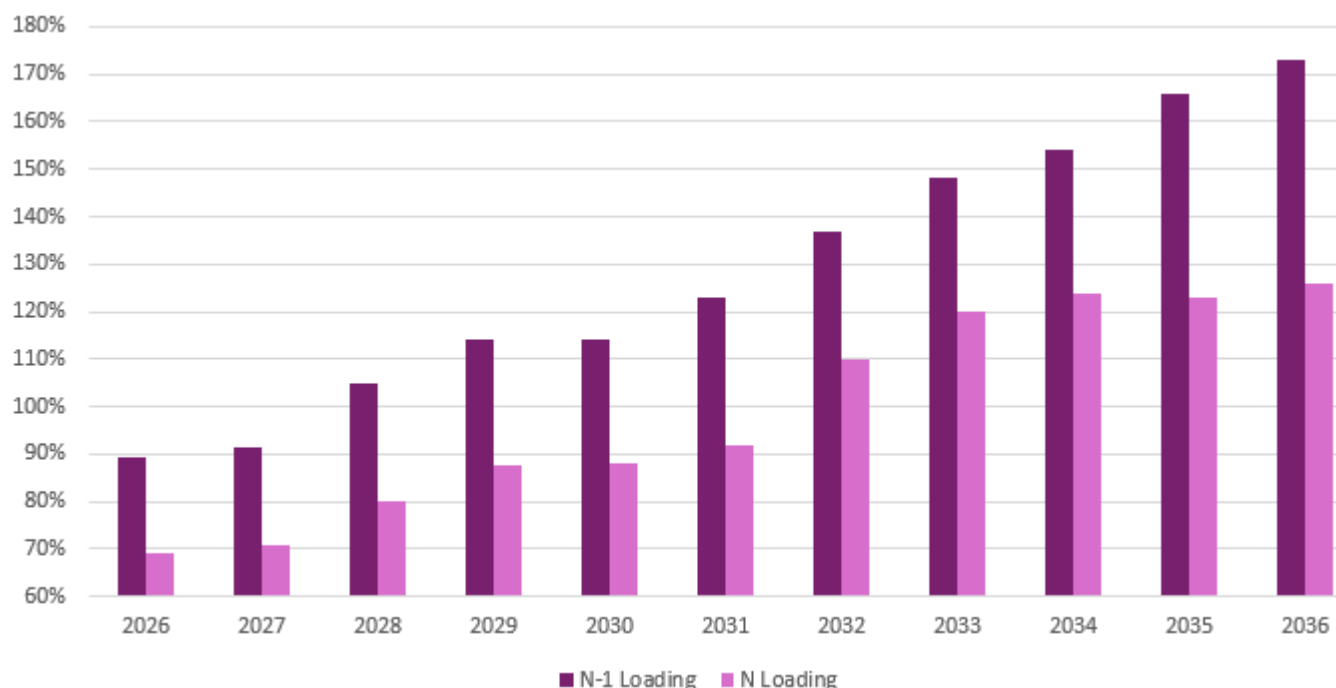
Figure 29 Thermal overloading of Keilor 500/220 kV A2 and A4 transformers
